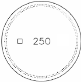
VIEW ON BASE SHOWING EMBOSSED MARKING STANDING AREA EMBOSSED WITH KNURLING.
